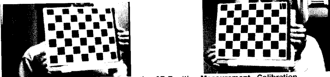
Figure 5-20. Illustrating 3D Position Measurement - Calibration
