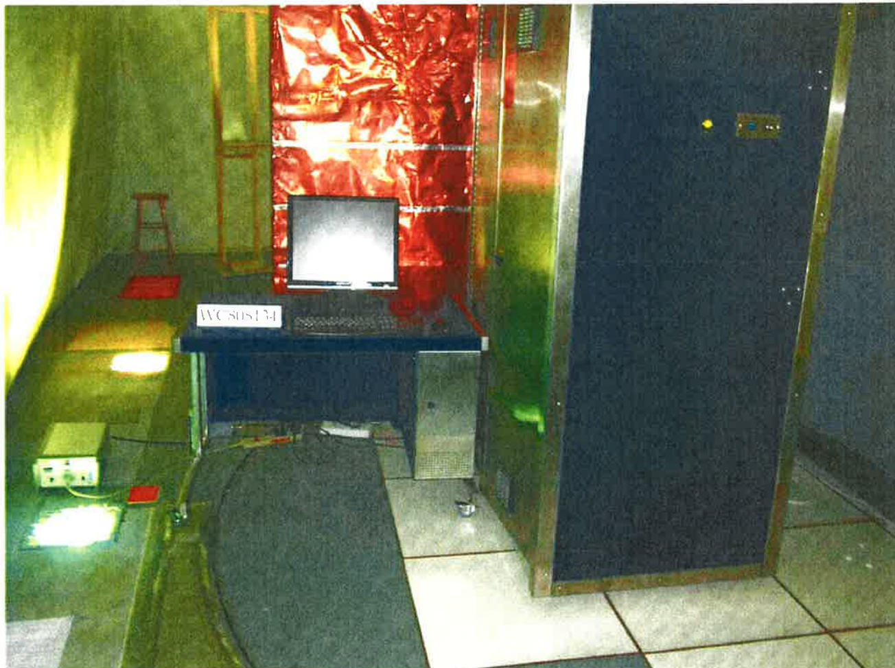
Test-setup photo(s): Conducted emission 150 kHz - 30 MHz
