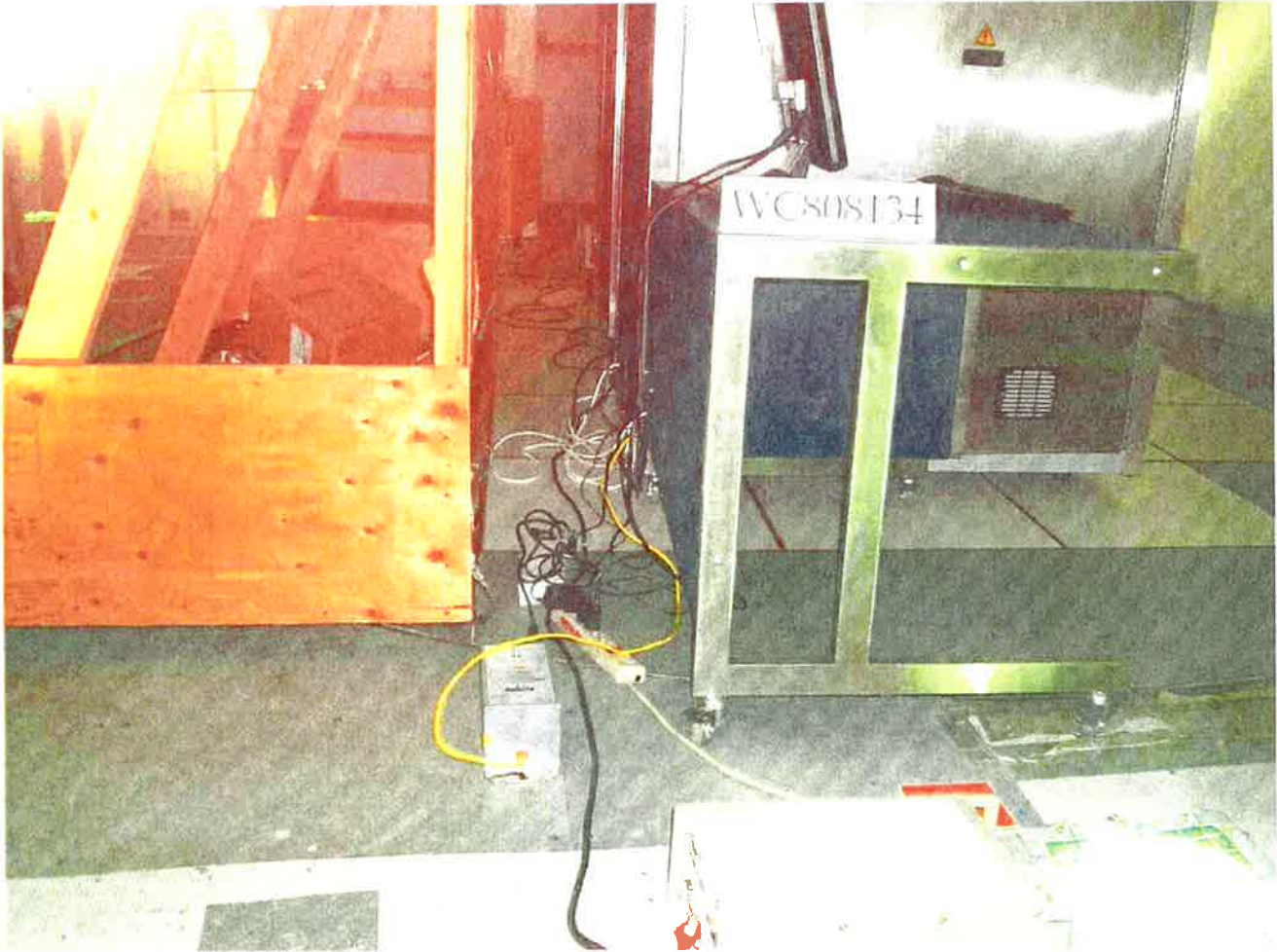
Test-setup photo(s): Conducted emission 150 kHz - 30 MHz
