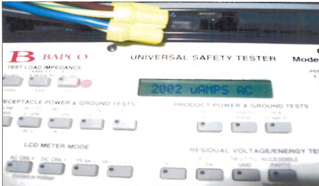
Close up of safety analyzer during testing leakage current
