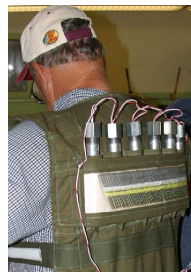
Figure 1 – Reproduction of typical body-worn explosive
