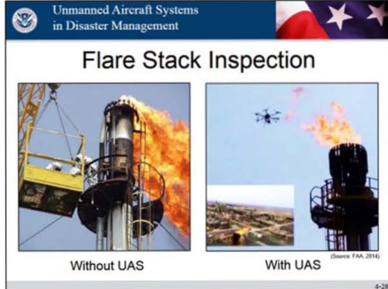
Slide 4-28. Flare Stack Inspection
