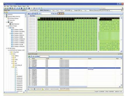
Figure 1: wear leveling in action. the same text message shows up multiple times because garbage collection has not yet happened
