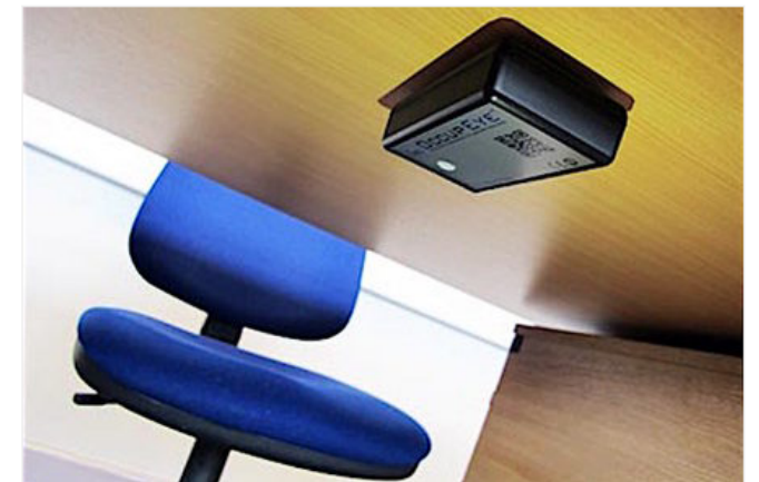
Eye spy OccupEye ... How the sensor box can be fitted to a desk
