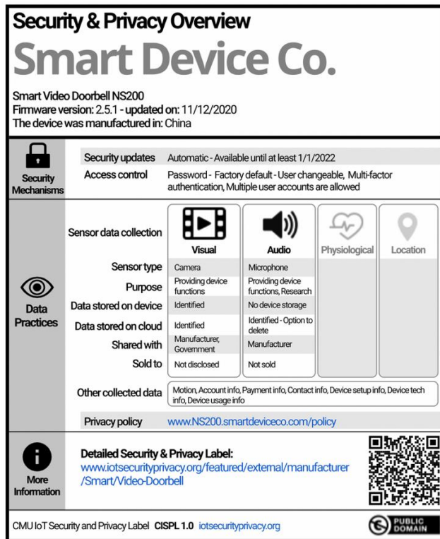
Fig. 1: Primary layer of the mock label in the CMU study. This layer should be printed on IoT product packaging and appear online alongside the product on retailer websites.
