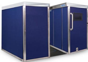
Backscatter AIT uses a narrow, low-energy x-ray beam that scans the surface of the body at a high speed. The machine then generates an image resembling a chalk etching with a privacy filter applied to the entire body. The image is displayed on a remote monitor for analysis to determine whether objects are present.
