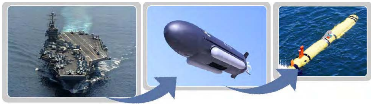
Figure 15 The cascading unmanned undersea vehicle concept deploys smaller UUVs with targeted payloads.
