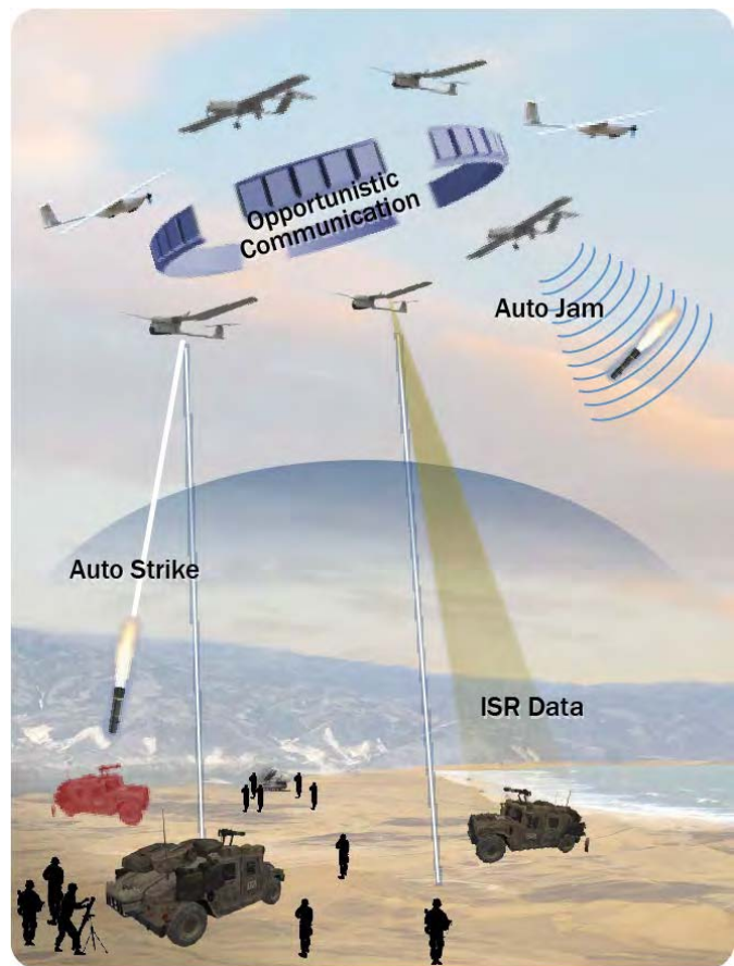
Figure 16 The concept for organic tactical ground vehicle support with an unmanned aircraft system would enable small units to anticipate threats, provide protection, and facilitate offensive action.
