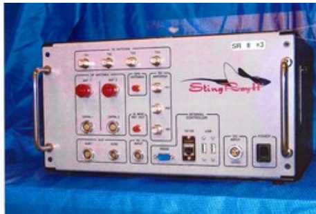
A Harris StingRay II, one of several devices dubbed 'stingrays.' U.S. Patent and Trademark Office
